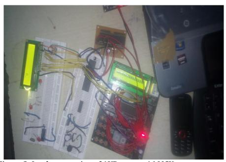
Figure 3: Implementat ion of AVR atmega16 MCU
